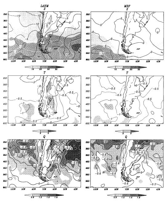
FIG. 4. (left panels) LAHM and (right panels) MRF 850-hPa 24-h forecast rmse (shaded) and bias (contoured) error for geopotencial height (m), temperature (K), and specific humidity (g kg<sup>-1</sup>).
