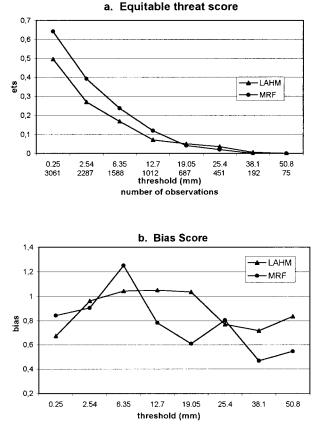
FIG. 13. The ETS and bias scores for LAHM and MRF 12–36-h forecast precipitation from Oct to Dec 2000.
